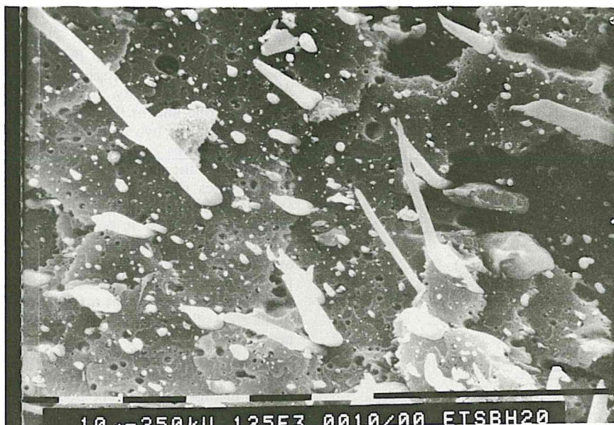
Fig. 8. SEM micrograph of extruded ribbon of PET/SBH 20%.
